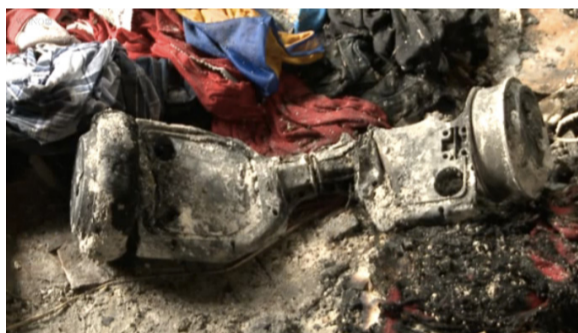
A Hover board that had caught fire while charging.
