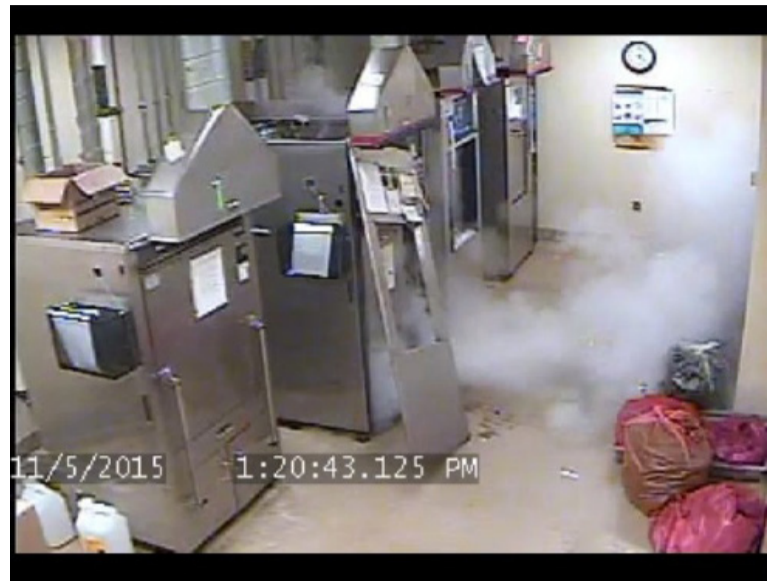
(Above) Steam release from DBI Autoclave incident
